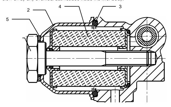
Slip off the used paper cartridge (4) from the long screw and discard it. You can now slip off the long screw from the aluminium cup: the sealing metal/rubber washer (5) on the base of the hex nut is now exposed and should be replaced with new one (D).
