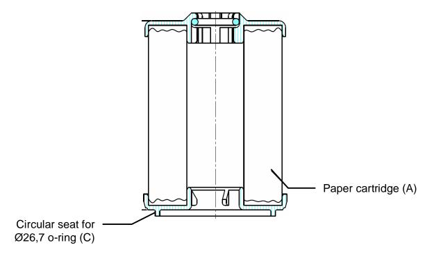
Put now the new paper cartridge (A) into the aluminium cup, so its black rubber o-ring (C) will face the filter body; then push the long screw into the aluminium cup and thru the paper cartridge. Finally put in place the new brown rubber o-ring (B), at the base of the aluminium cup.
